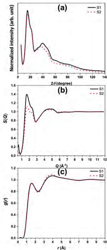
Fig. 2. (a) GIXS patterns, (b) total structure factor,  $S(Q)$ , and (c) pair distribution function  $g(r)$  of TaO<sub>x</sub> thin films with  $5 \times 10^{-5}$  Pa (S1) and  $1 \times 10^{-2}$  Pa (S2) oxygen partial pressures.
