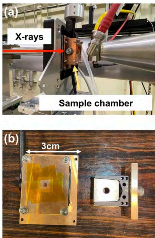
Fig. 3. (a) Humidity-conditioning sample chamber and (b) sample mount.
