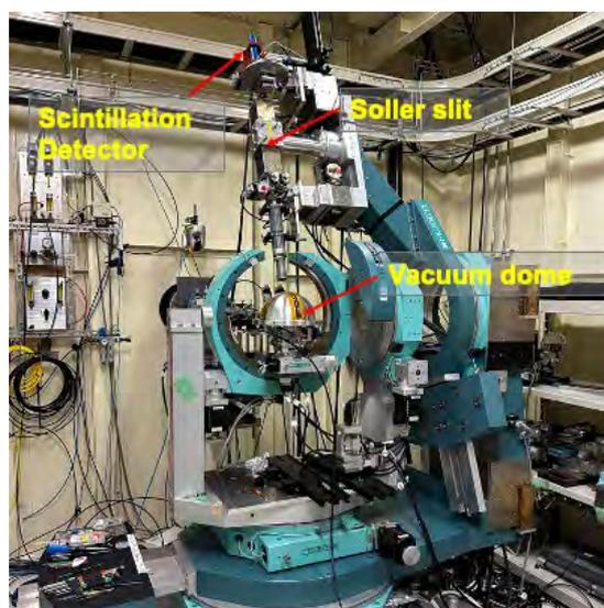
Fig. 1. Grazing-incidence X-ray scattering (GIXS) setup on the versatile multi-axis diffractometer installed at BL19B2 EH2.
